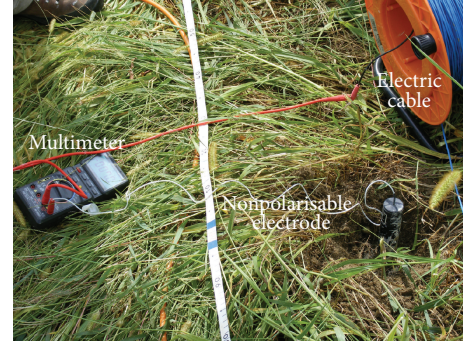
FIGURE 1: Instrumentation for SP measurement [33].
