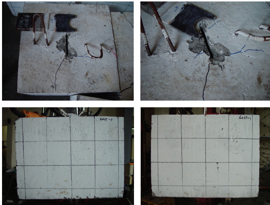
FIGURE 10: Failure mode of specimen PO-6015-R (Type IV).
