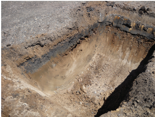
FIGURE 4: Example test pit showing, from top to bottom, typical soil profile: residual gray base aggregate, brown silty sand, black organic silt, brown silty sand.
