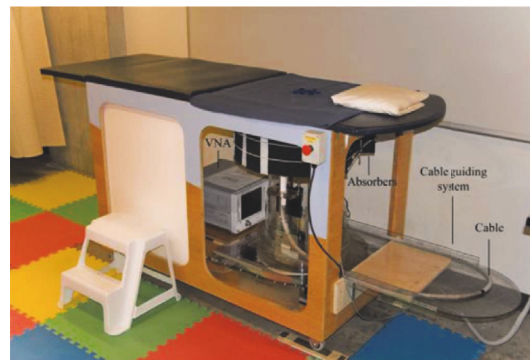
FIGURE 24: TSAR prototype system in Calgary University [28]. Image from Bourqui et al. 2012, under the Creative Commons Attribution License.
