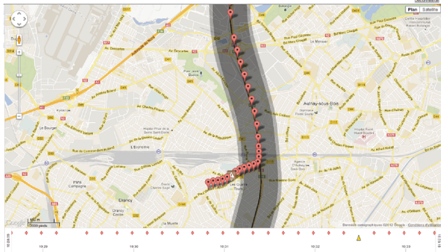
FIGURE 6: Real-case example where an alert is triggered shortly after a mobile leaves the corridor.
