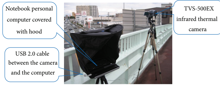
FIGURE 1: The infrared thermal camera and the notebook personal computer covered with the hood on a pedestrian bridge.
