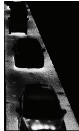
FIGURE 12: An image in lane 2 after final optimum gamma transformation.
