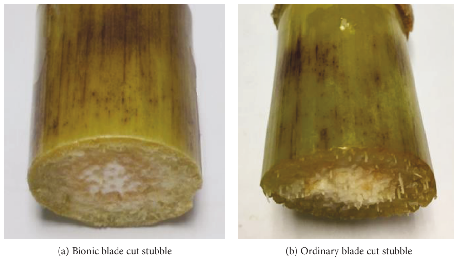
FIGURE 9: Comparison of cut stubble using both bionic and ordinary blades.
