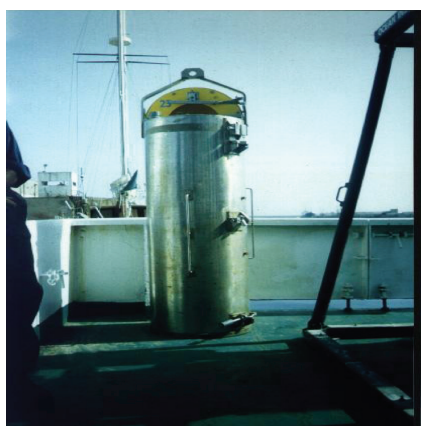
FIGURE 2: Seawater sampler (IAEA).
