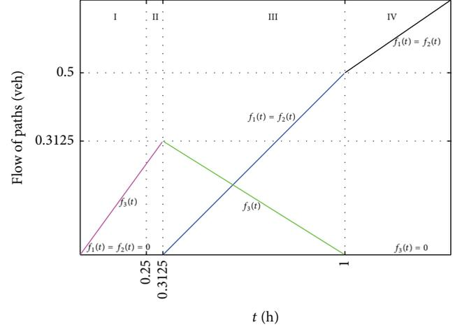
FIGURE 3: Equilibrium flow of the dynamic network ( $t(\text{h})$  versus flow (veh)).
