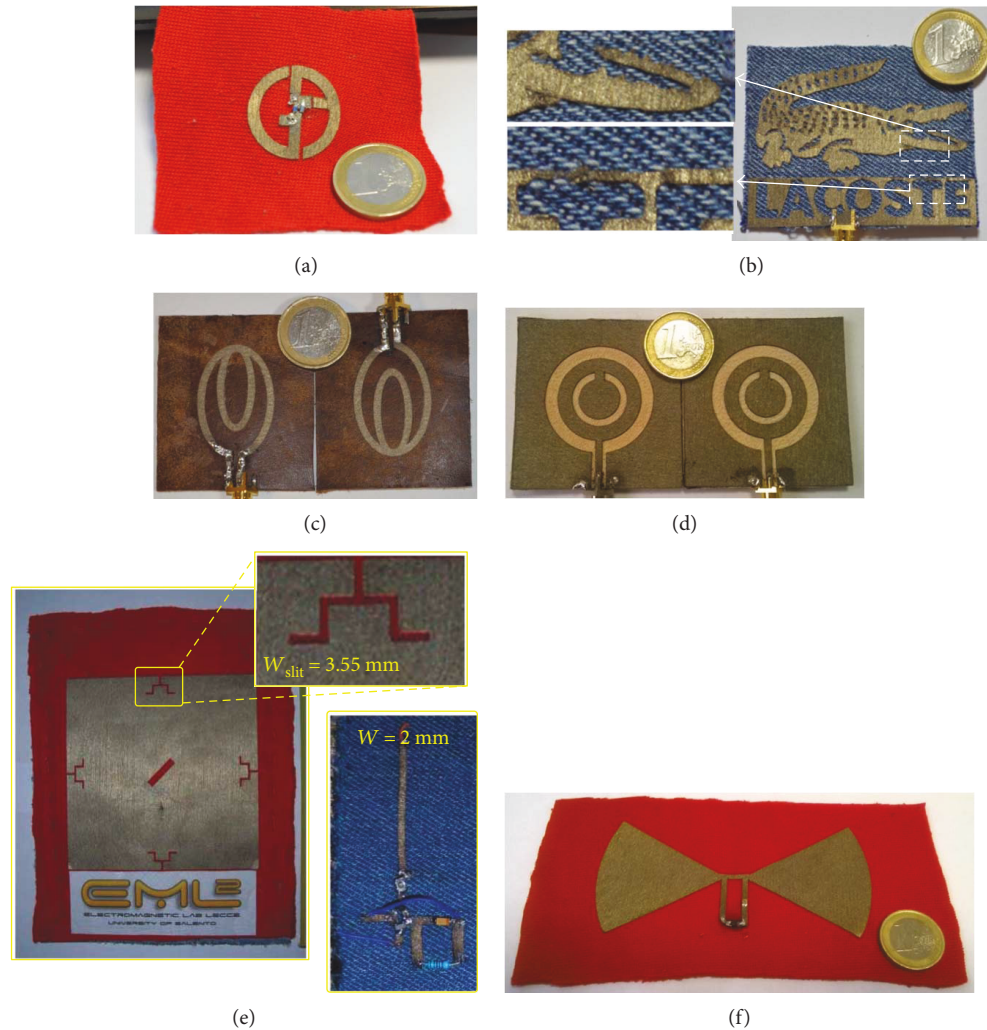
FIGURE 6: Wearable antenna prototypes realized by using for the conductive part's adhesive conductive nonwoven fabrics. (a) An antenna which mimics the shape of Giorgio Armani's logo. (b) An antenna which mimics the shape of Lacoste's logo. (c) Wearable resonators having an elliptical loop geometry. (d) Wearable resonators exploiting a complementary split ring resonator geometry. (e) Wearable rectenna. (f) Bow tie-like UHF RFID tag.
