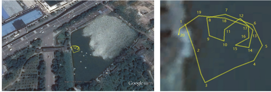
FIGURE 12: Navigation trajectory of the sail-assisted USV.
