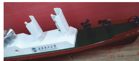
FIGURE 7: The wind sensor system of the SUICS.
