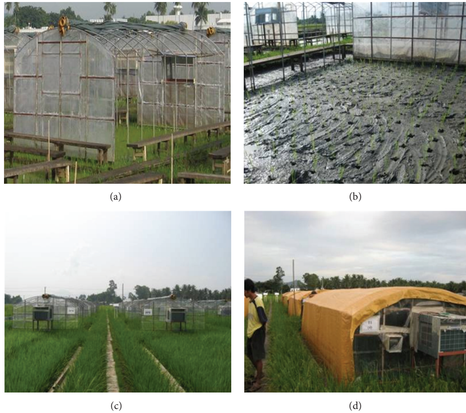
FIGURE 1: The actual setup of a field chamber located at the IRRI farm. (a) Single chamber; (b) inside of chamber with rice seedling; (c) profile of the chamber systems in field. (d) Chamber covered by canvas after 6PM.
