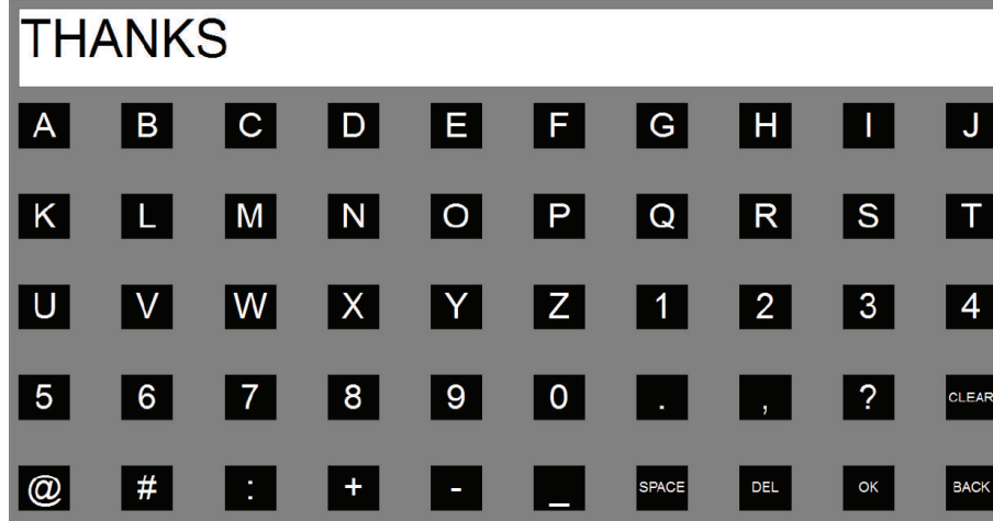
FIGURE 6: The GUI of the P300-based speller that is used for text input. Fifty buttons arranged in a 5 by 10 stimuli matrix corresponding to 45 characters and 5 function keys. “CLEAR” is used to clear all of the input characters, “SPACE” is used to input a space, “DEL” is used to delete the last input character, “OK” is used to return to the mail client interface with the input text, and “BACK” is used to cancel the input text and return the user to the mail client interface.
