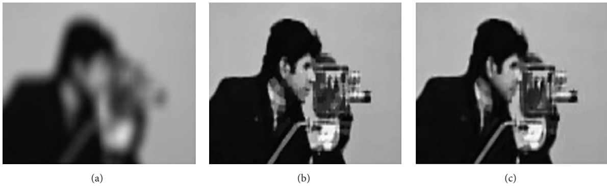
FIGURE 2: (a) Blurred input data, MSSIM = 0.032 . (b) Solution-driven adaptive TV, MSSIM = 0.866 . (c) Solution-driven adaptive generalized TV, MSSIM = 0.868 .
