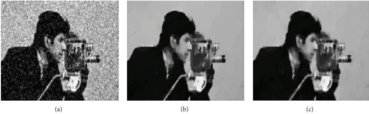
FIGURE 1: (a) Noisy input data, MSSIM = 0.327. (b) Solution-driven adaptive TV, MSSIM = 0.812. (c) Solution-driven adaptive generalized TV, MSSIM = 0.822.
