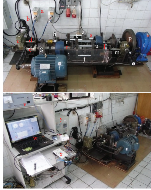
FIGURE 4: Experimental setup of prototype DBVCVT and test rig. (a) DC servo motor controllers; (b) DC servo motor (secondary pulleys); (c) worm gearbox of DC servo motor (secondary pulleys); (d) power screw mechanism (secondary pulleys); (e) integral torque and speed sensors (primary pulleys); (f) three-phase AC motor; (g) spring; (h) load cell (secondary pulleys); (i) variator 1; (j) variator 2; (k) inverse differential gearbox; (l) load cell (primary pulleys); (m) power screw mechanism (primary pulleys); (n) worm gearbox of DC servo motor (primary pulleys); (o) DC servo motor (primary pulleys); (p) flywheel; (q) magnetic powder dynamometer; (r) input shaft; (s) output shaft; (t) synchronous shift fork (secondary pulleys); (u) synchronous shift fork (primary pulleys); (v) dynamometer controller; (w) control program; (x) programmable ECU; (y) inverter for AC motor; (z) optical sensor.
