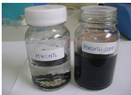
FIGURE 3: The typical image of MWCNTs-COOH was well dispersed in water after 30-minute ultrasonic vibration.
