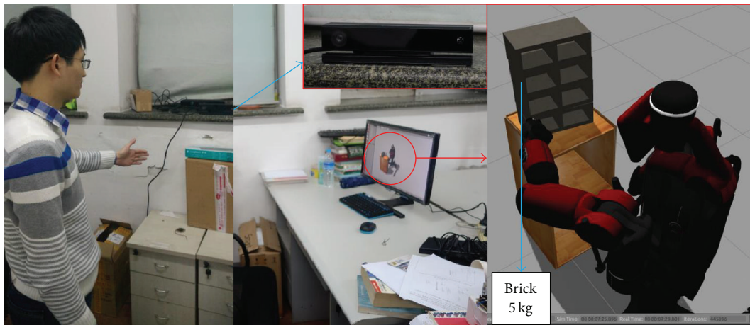
FIGURE 10: Experimental setup for human and Baxter robot collaboration intuitively and compliantly in teleoperation scenario. The virtual Baxter robot environment is based on ROS and gazebo [58]. Four bricks are put on the shelf and their total weights are modified to 5 kg. Baxter robot is supposed to move the four bricks with different arm configurations.
