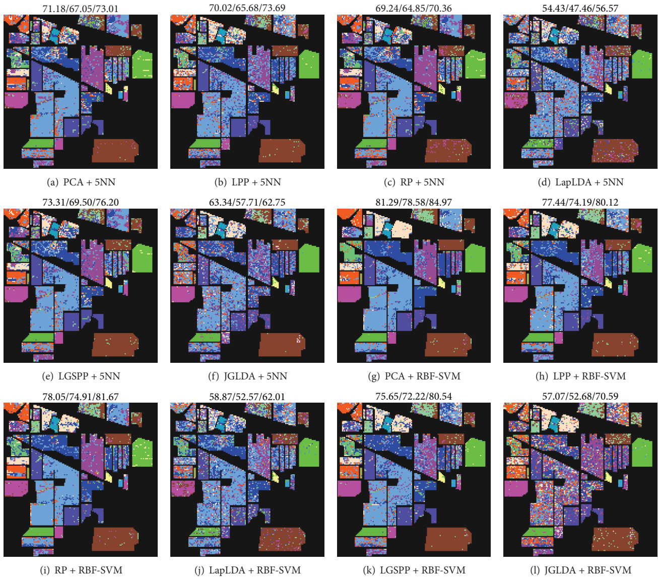
FIGURE 4: RGB composition and classification map for AVIRIS Indian Pines. The overall accuracy/kappa coefficient/average accuracy are also included at the top of each map, respectively.
