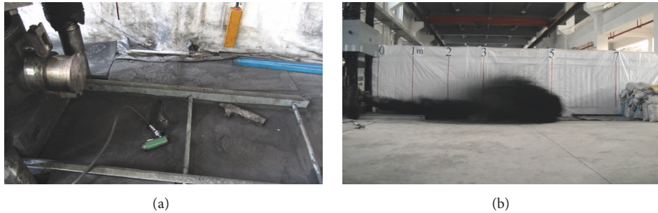
FIGURE 9: A photograph of the outburst simulation experiments ((a) Xuehu: weak outburst, 0.216 MPa, CO 2 ; (b) Fenghui: strong outburst, 0.346 MPa, CO 2 ).
