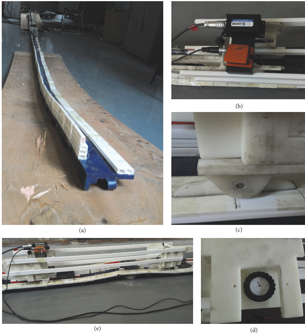
FIGURE 10: (a) Shape of the scraper conveyor; (b) the two sensors installed in the shearer body; (c) the supporting sliding shoe; (d) the walking wheel; (e) the shearer prototype.
