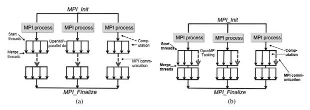
Fig. 2. Two different hybrid models in GTS using standard OpenMP worksharing (a) or the newly introduced OpenMP tasks to execute MPI communication while performing computation (b). (a) Original MPI/OpenMP hybrid model. (b) MPI/OpenMP hybrid model using OpenMP tasks to overlap MPI.
