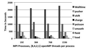
Fig. 3. Evaluation of MPI/OpenMP hybrid model with GTC on Hopper.
