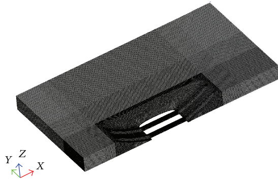
FIGURE 14: Hydroplaning computational domain mesh.
