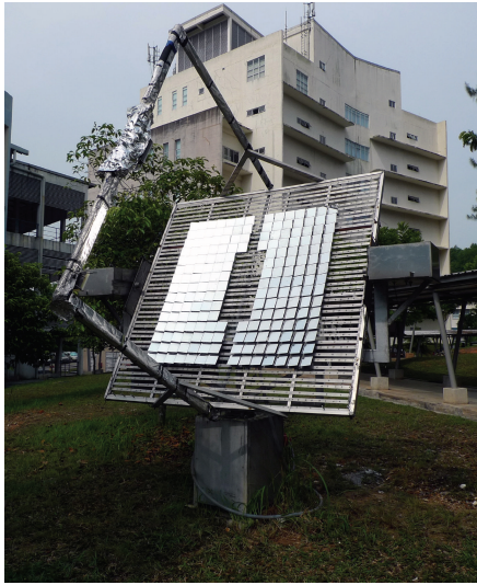
FIGURE 3: A prototype of nonimaging planar concentrator (NIPC) in the campus of Universiti Tunku Abdul Rahman (UTAR), Malaysia.
