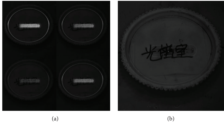
FIGURE 6: Images in (a) are acquired by our polarization CCD camera at polarization orientations of 0^\circ , 45^\circ , 90^\circ , and 135^\circ , respectively. (b) is the result through our reflected highlight removing method, where only tiny residual can be found.
