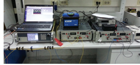
FIGURE 14: Photo of the experimental setup: two power amplifiers emulate the PV modules and one power amplifier emulates the load.
