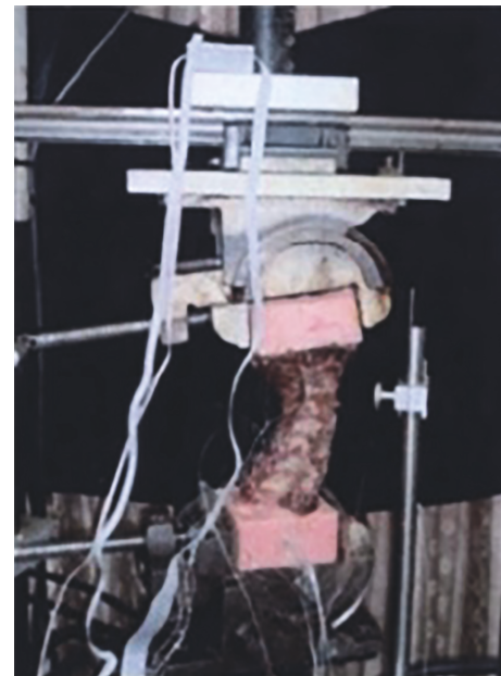
FIGURE 6: The maximum allowable acceleration of the cervical spine measured with the Zwick Roell BX1-EZ005.
