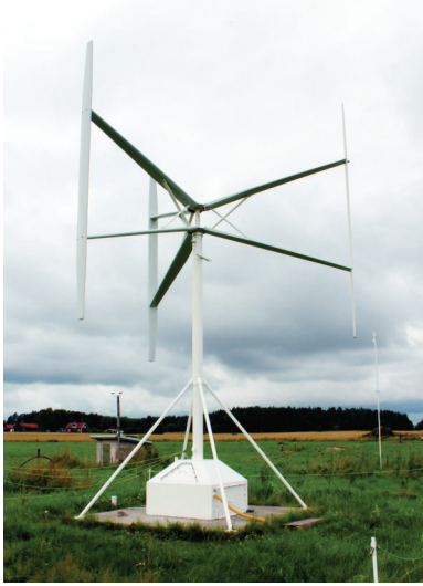
FIGURE 1: 12 kW vertical axis wind turbine designed and constructed at Uppsala University.
