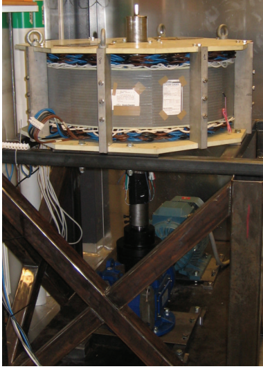
FIGURE 4: Permanent magnet synchronous generators used in the experimental setup.
