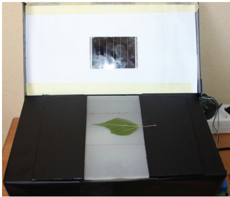
FIGURE 3: The layout of the opal glass used for diffusing the parallel reflected light.
