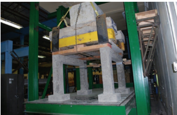
FIGURE 2: Experimental setup of the model on the shake table.
