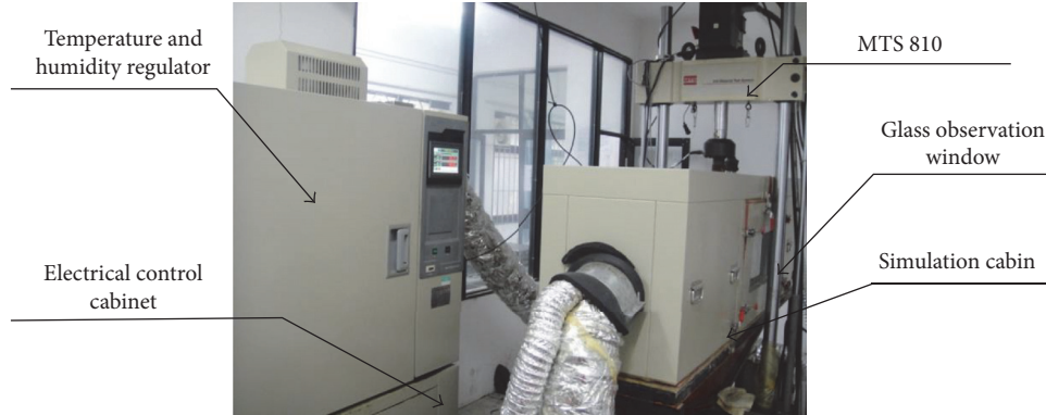
FIGURE 10: Hot-wet environment simulation and control system.
