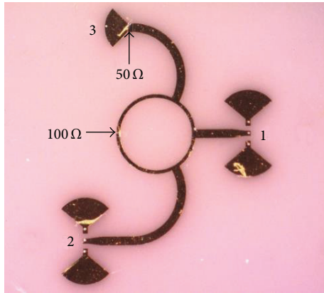
FIGURE 10: Microphotograph of the Wilkinson power divider/combiner.
