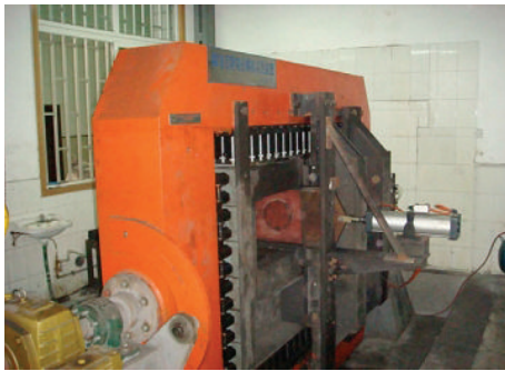
FIGURE 2: Large-scale simulation test system of coal and gas outburst.
