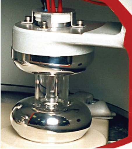
FIGURE 2: Electrooptic BGO voltage sensor in 170 kV gas-insulated switchgear. The BGO crystal is inside the transparent insulator tube between the electrodes at high voltage (bottom) and ground potential (top). The crystal is operated in a reflective mode with optical fiber cables (red) guiding the light to and from the ground potential side.
