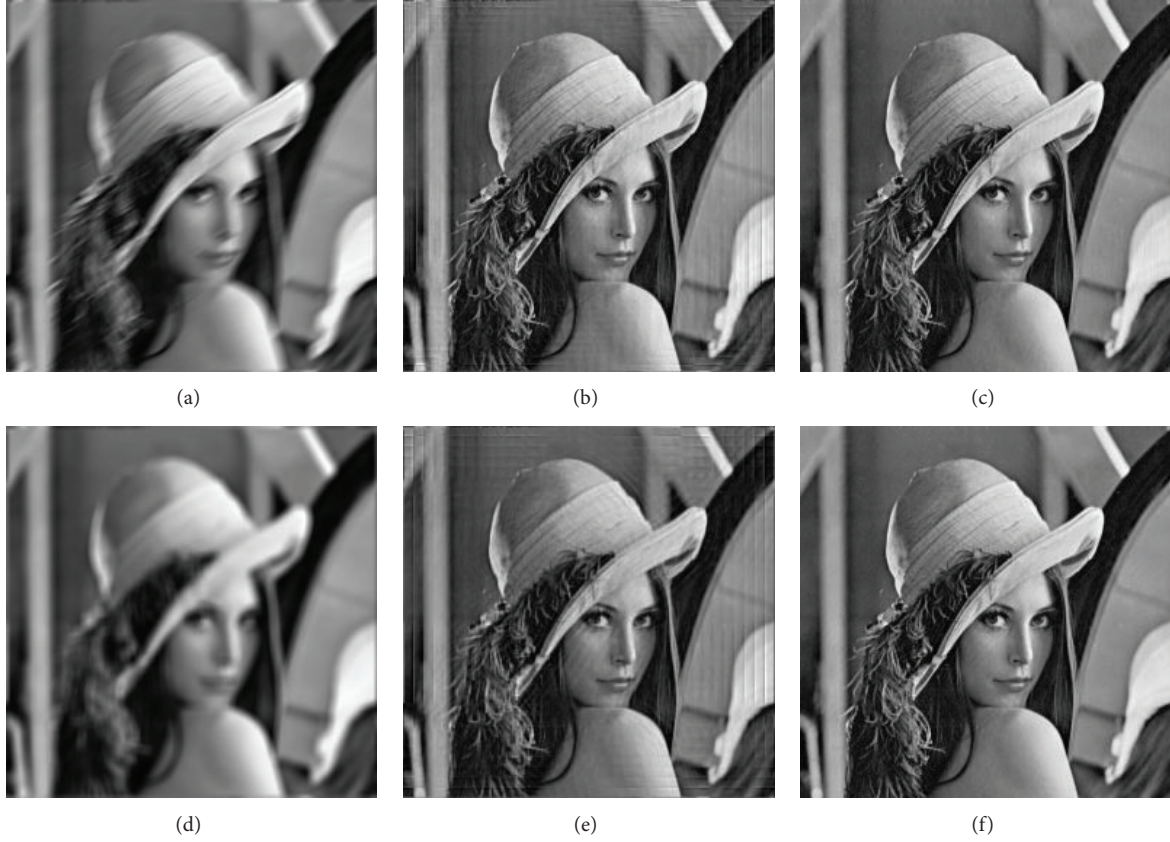
FIGURE 5: Comparison with SBI method. First column: motion blurred image and uniform blurred image. Second column: images deblurred by SBI. Third column: images deblurred by PSBI.
