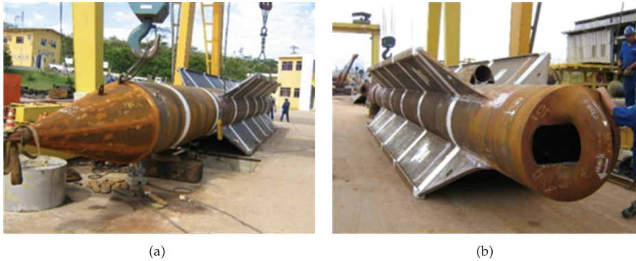
Figure 1: Typical torpedo anchor with four flukes: (a) conical tip and (b) top with detail of the padeye.
