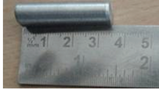
FIGURE 2: Typical specimen of AA 6351-fly ash reinforced MMC.
