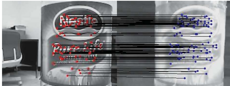
Fig. 8. Successful fine motion alignment between template (left) and left gripper camera view (right) (best viewed in color).
