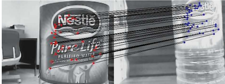
Fig. 7. Object recognition: a successful match between template (left) to current gripper camera view (right) after gross motion and visual alignment.
