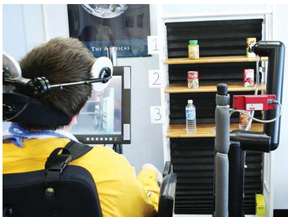
Fig. 9. Experimental setup with single switch scanning. P5 used Cross Scanner [35] single switch scanning software and activated the scanning with a head switch.
