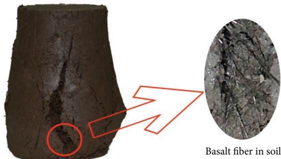
FIGURE 5: Failure form of basalt fiber reinforced soil sample.
