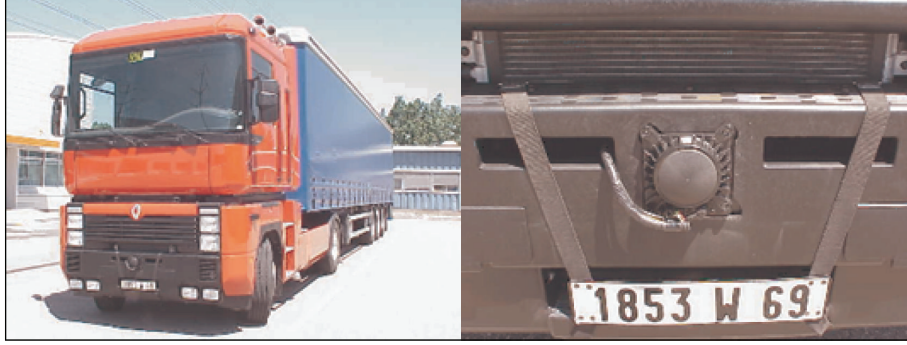
FIGURE 1: Radar installed on the Renault Magnum truck.
