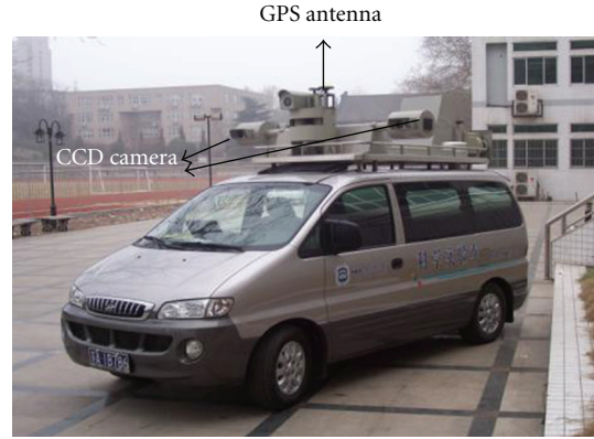
(a) The appearance of vehicle-borne mobile mapping system
