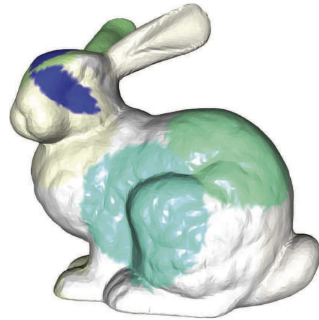
FIGURE 5: The patches of the bunny model by choosing N_1 = 1000 , N_2 = 200 , and N_3 = 600 . Patches are shown by different colors, and overlapping regions are shown by blue.
