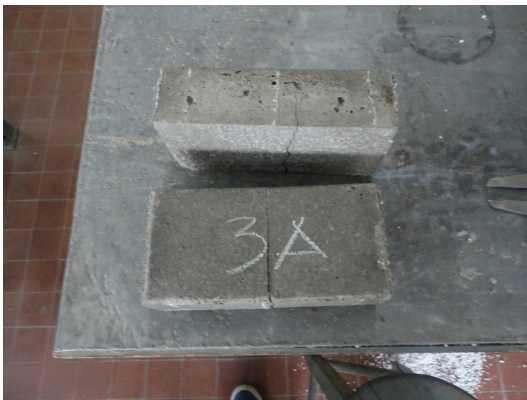
FIGURE 2: Resulting cracks in the brick under Tensile test.
