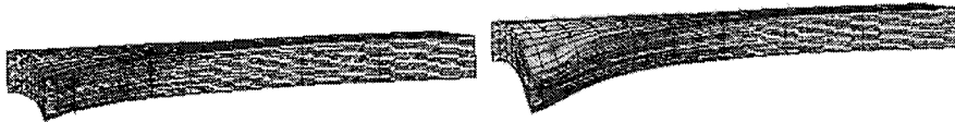
Figure 10. Final delamination contours of a [0/90]_{3S} laminate impacted at 20 °C (left) and -150 °C (right). Impact energy: 3 J.
