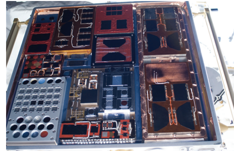
FIGURE 9: Sun looking face of the Passive Experiment Container (PEC) containing passive material samples and cells as flown on Materials International Space Station Experiment 7 (MISSE7). Solar cells can be denoted by the wires to attach to the measurement circuitry of the Forward Technology Solar Cell Experiment II (FTSCE II) (image courtesy of NASA).
