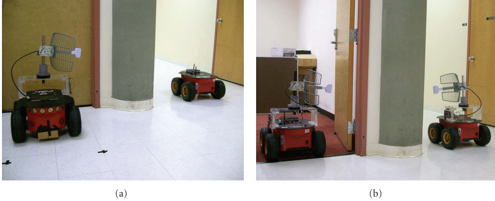
FIGURE 12: (a) Pioneer robots gathering data at the basement of the ECE building at UNM with the transmitter using an omnidirectional antenna and the receiver using a directional one. (b) Pioneer robots using directional antennas for both transmission and reception.
