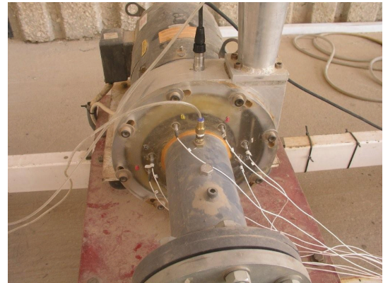
FIGURE 4: Measurements of pressure fluctuations: model pump.
