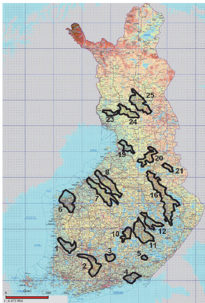
FIGURE 18: Glaciotectonic features occur noticeably in these hummocky moraine fields with original field numbers. The fields are presented as modified after Mäkinen et al. [22]. Subglacial thrust features are quite widely spread in Finland.
