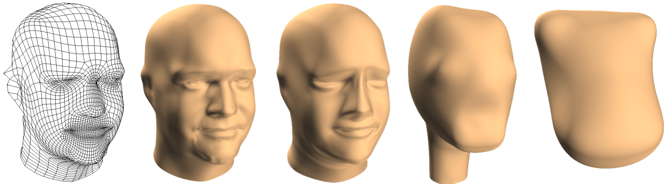
Figure 4: Unconstrained fairing of a complex subdivision surface (6975 dofs). Solution until convergence took 152 iterations (20m5s) using the nonlinear minimizer. We show the original model, intermediate meshes at 20 and 100 iterations and the final mesh. Even though the model is topologically equivalent to a disk, the gradient \nabla(E_{\text{ad}}^{\text{b}}) disappears for the right-most mesh.
