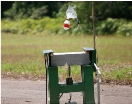
FIGURE 2: Field blast test setup.
