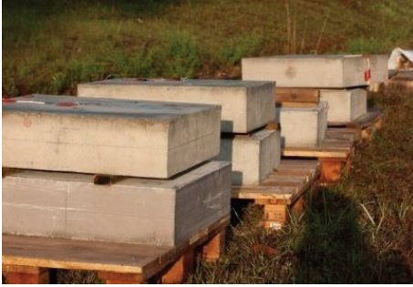
FIGURE 1: Reinforced concrete test panels.
