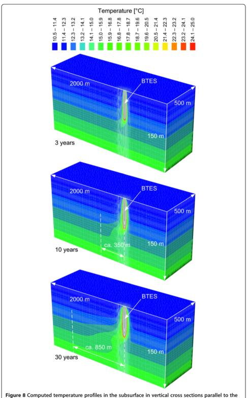
Figure 8 Computed temperature profiles in the subsurface in vertical cross sections parallel to the aquifer flow direction. After 3, 10, and 30 years of operation; vertical exaggeration,  $\times$ 5.
