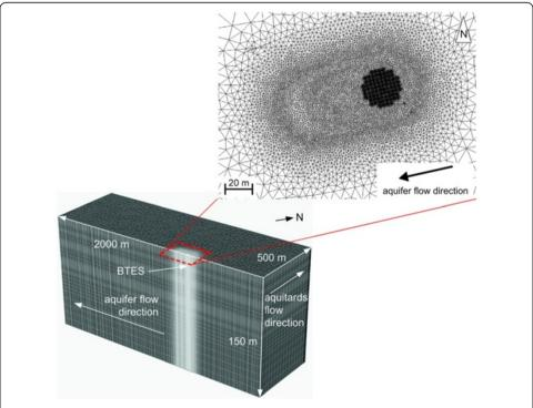
**Figure 5 Model meshing and layer dimensions of the 3D finite element mesh.** Vertical cut through the middle of the thermal storage along the aquifer flow direction; vertical exaggeration, ×5.
