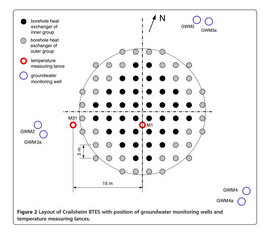
and M31 (see Figure 2). Both measuring lances record temperatures of the solid underground up to a depth of 80 m.
