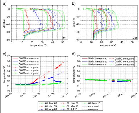
**Figure 7 Measured and computed underground and groundwater temperatures.** Measured and computed underground temperatures at measuring lances M1 (a) and M31 (b) and measured and computed groundwater temperatures at wells GWM2/a, GWM3/a, and GWM4/a at 20-m depth (c) and 80-m depth (d).
